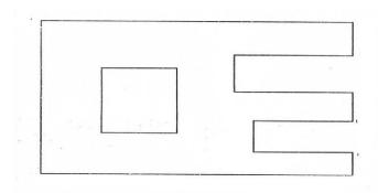
12. Copy the given sketch to 1:1 scale and dimension adopting unidirectional system with parallel dimensioning method.
