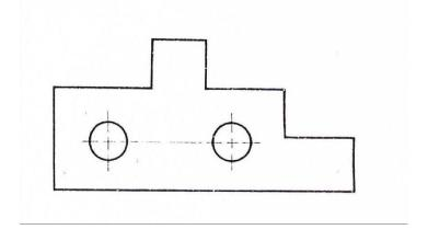
10. Copy the given sketch to 1:1 scale and dimension adopting unidirectional system with chain dimensioning method.
