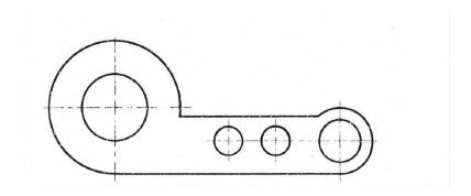
11. Copy the given sketch to 1:1 scale and dimension adopting unidirectional system with combined dimensioning method.
