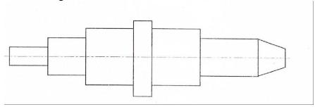
9. Copy the given sketch to 1:1 scale and dimension adopting aligned system with progressive dimensioning method.
