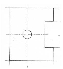
13. Copy the given sketch to 1:1 scale and dimension adopting aligned system with chain dimensioning method.
